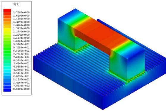
a) LTFRM with core branch's height of 5 mm
