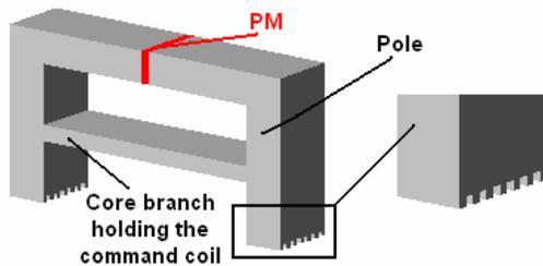
Fig. 4. The iron core of the mover.
