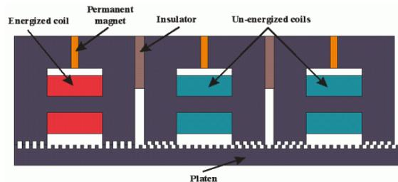
Fig. 2. The modular double salient PM linear motor.
