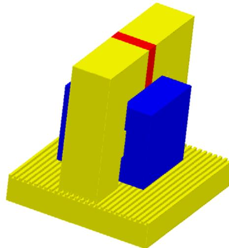
Fig. 7. The analyzed LTFRM structure with PMs on the mover.
