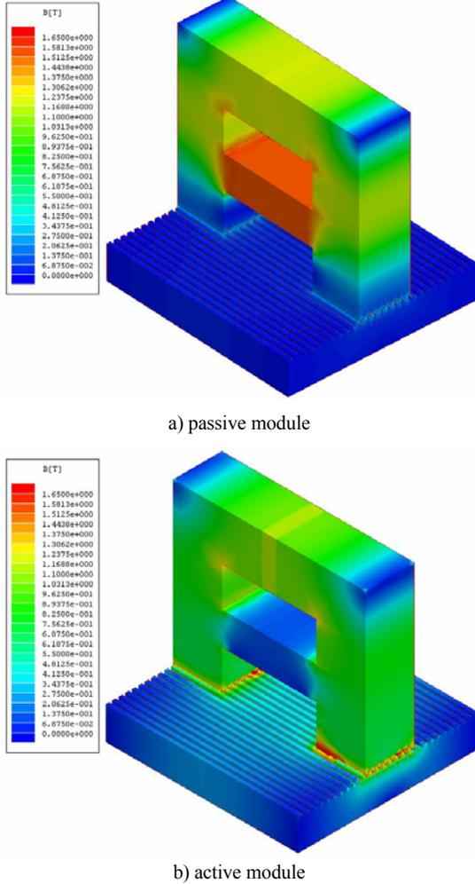
Fig. 7. The flux density distribution obtained via 3D FEM analysis for the LTFRM with PMs on the mover on the mover
