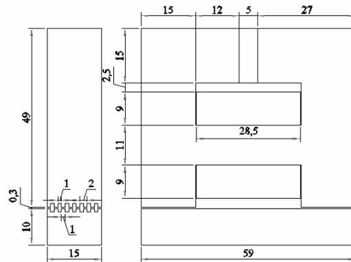
Fig. 6. Main sizes of proposed linear TFM module (lateral and frontal view)
