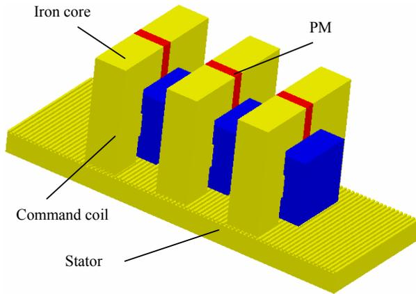
Fig. 3. The proposed modular linear machine.
