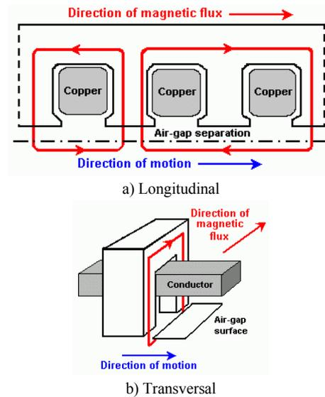
Fig. 1. Magnetic flux orientation in electrical machines.
