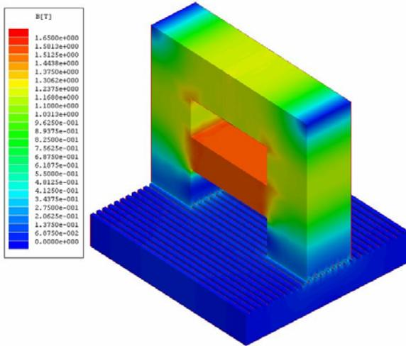
Fig. 13. The flux density distribution in a passive module obtained via 3D FEM analysis.
