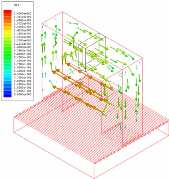
Fig. 12. The flux density vector in a passive module obtained via 3D FEM analysis.
