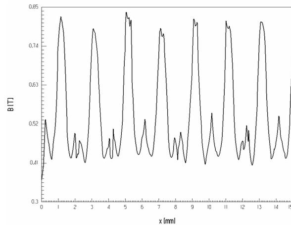
Fig. 11. The air-gap flux density variation vs. length for unaligned teeth with supplied coil.
