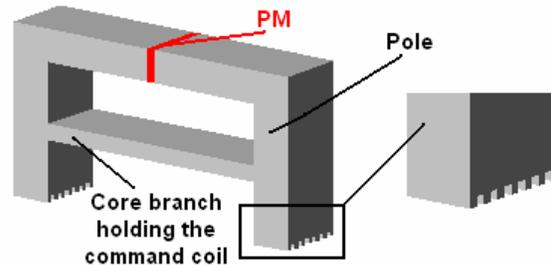
Fig. 3. The iron core of the mover.
