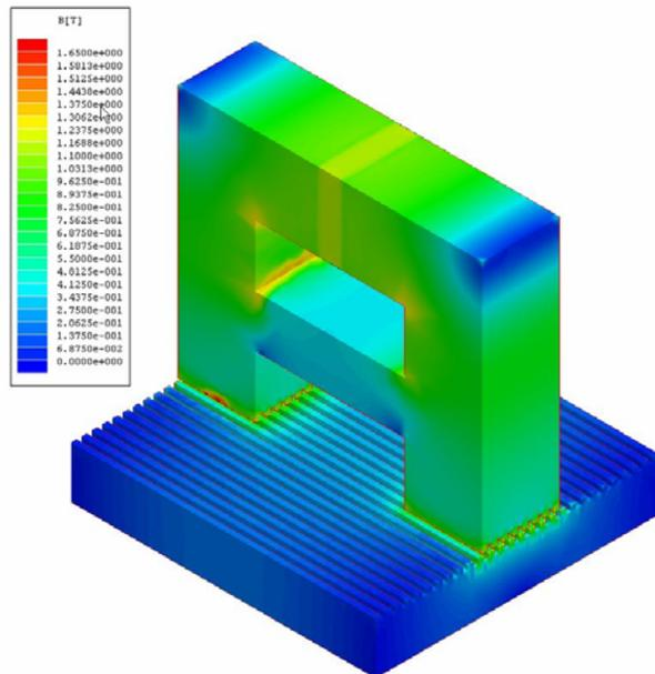
Fig. 10. The flux density distribution in an active module obtained via 3D FEM analysis.
