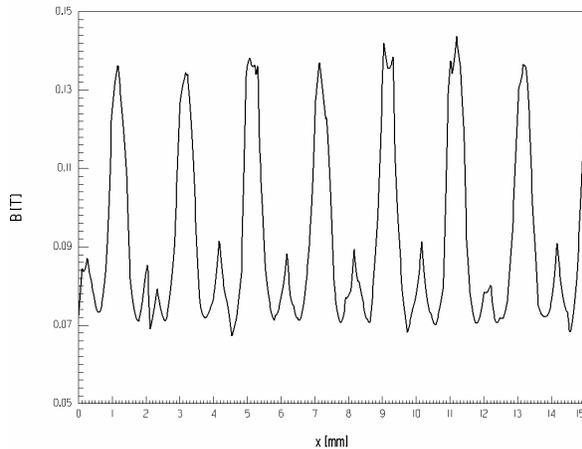
Fig. 14. The air-gap flux density variation vs. length for aligned teeth with unsupplied coil.
