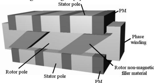
Fig. 1. A TF machine with passive rotor and permanent magnets in the stator.
