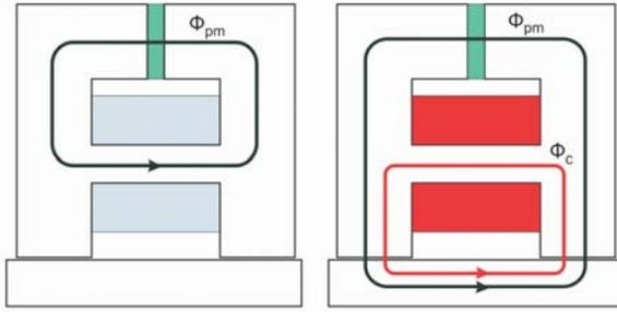
Fig. 4. The working principle of the linear machine.
