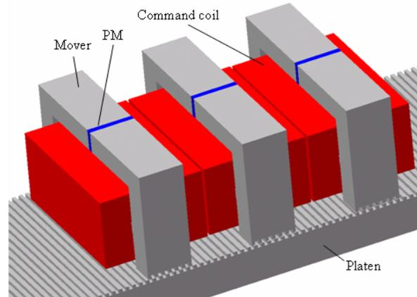
Fig. 2. The proposed modular linear machine.
