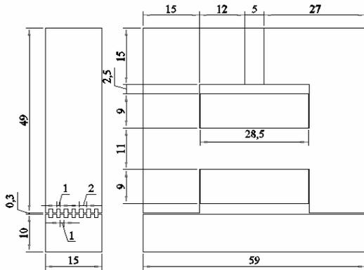
Fig. 5. Main sizes of proposed linear TFM module: a) lateral view; b) frontal view.
