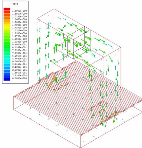
Fig. 9. The flux density vector in an active module obtained via 3D FEM analysis.
