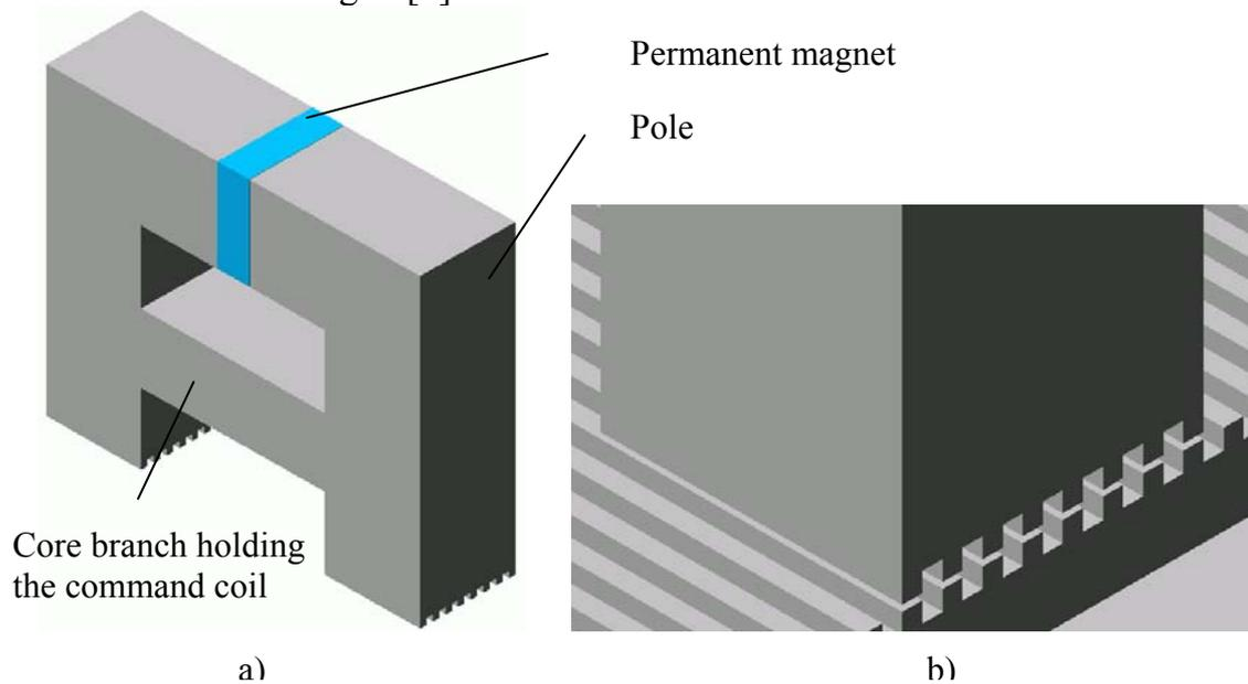
Fig. 2. The iron core of the mover: a) whole structure; b) toothed part.
