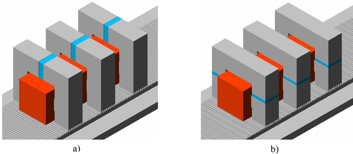
Fig.1. Two structures of linear transverse flux reluctance machine
