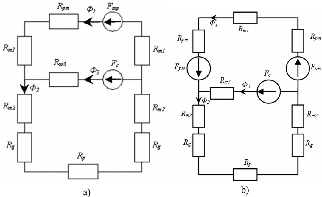
Fig.4. The equivalent magnetic circuit of the two machines:
