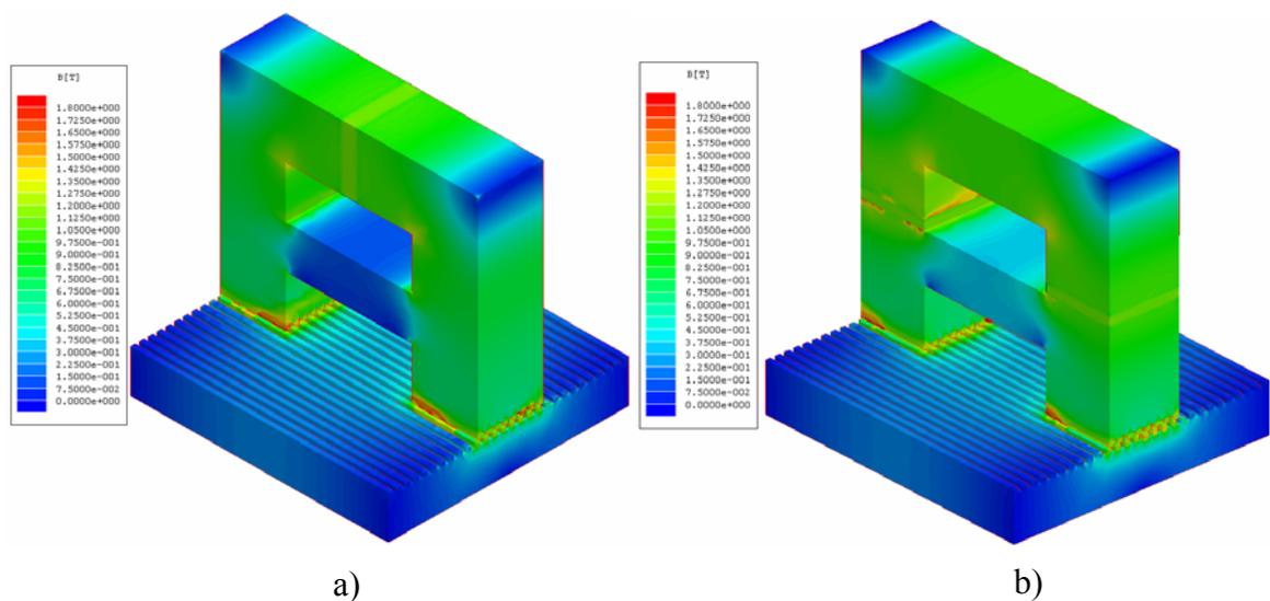
Fig. 6. The flux density distribution obtained via 3D FEM analysis:
