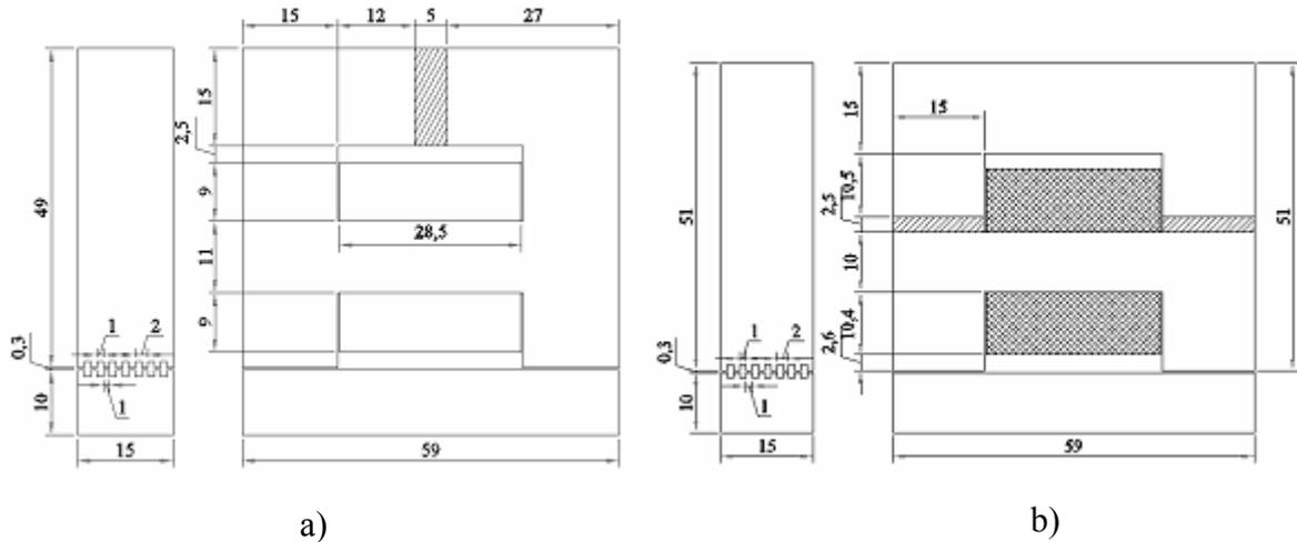
Fig.5. Lateral and frontal view of the proposed linear TFM's:
