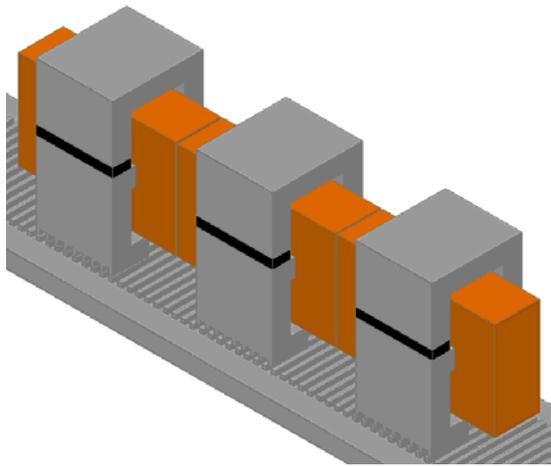
Fig. 3. The linear transverse flux reluctance machine with permanent magnets with enlarged teeth surface.
