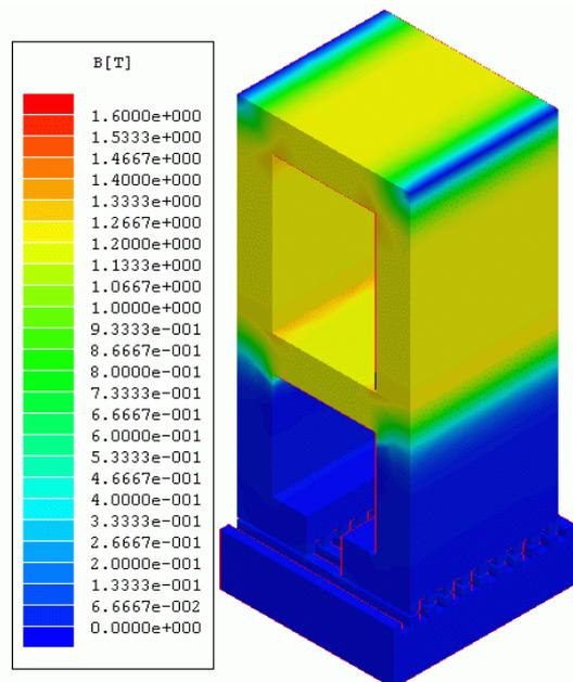
Fig. 7. Distribution of the flux density in a passive module of the machine having
