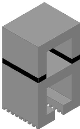
Fig. 4. Iron core with permanent magnets of a module of the linear transverse flux reluctance machine with enlarged teeth surface.
