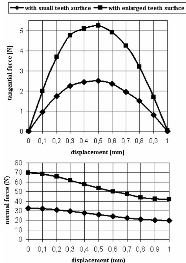
Fig. 9. The variation of the forces versus the module shifting for the two presented machines:
