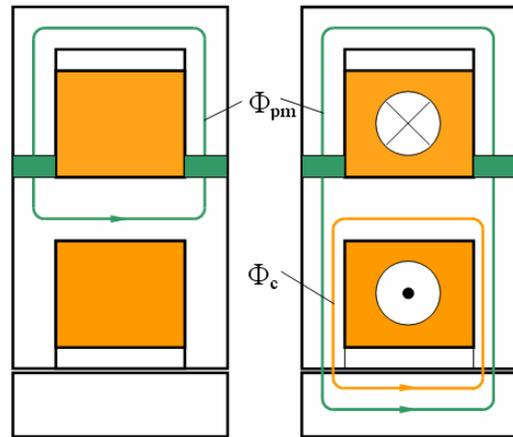
Fig. 2. The working principle of the permanent magnet linear transverse flux reluctance machine.
