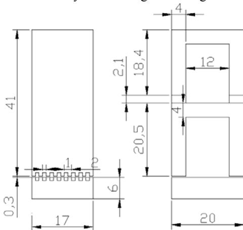
Fig. 5. Main sizes of linear TFM module with small teeth surface: a) lateral view; b) frontal view.
