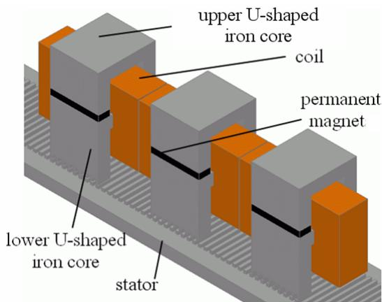
Fig. 1. The linear transverse flux reluctance machine with permanent magnets.
