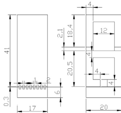
Fig. 6. Main sizes of linear TFM module with enlarged teeth surface: a) lateral view; b) frontal view.
