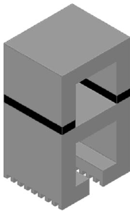
Fig. 4. Iron core with permanent magnets of a module of the linear transverse flux reluctance machine with enlarged teeth surface.
